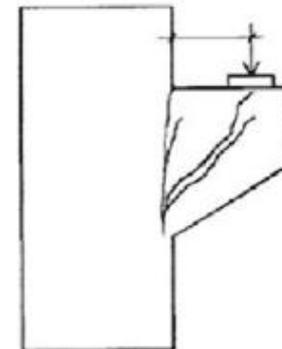
(b) Concrete crushing on strut
