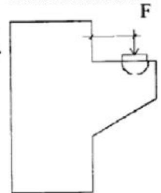
(f) Concrete crushing under the bearing pad
