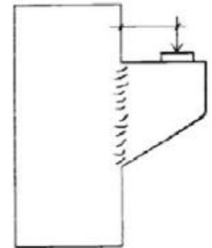
(c) Shear at the interface between corbel and column
